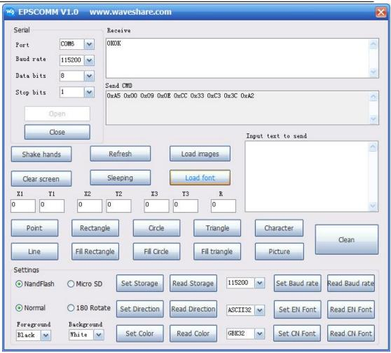
3. Click the button Load image. Then, the state indicator on the e-Paper will flicker 3 times, indicating the importation starts. When finished, the state indicator will flicker 3 times again and the e-Paper module will return the message "OK", indicating that the importation of image(s) is completed successfully.
